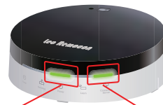
[Power] 指示灯 [Connecting Server] 指示灯
